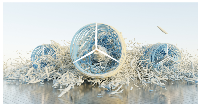
Figure 3: Results from neutral ABL study. Shown is an isosurface of q -criterion, colored by the x -component of velocity. Note that while there is a considerable amount of ‘noise’ near the turbines, the wake maintains a straight-back structure.
