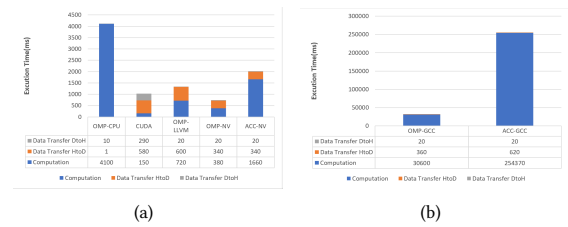
Figure 3: Kernel execution time of stream cluster using different parallel models and compilers, a) total execution time for LLVM, NVCC and NVC compilers, b) total execution time for gcc compiler. OMP-CPU version is compiled by LLVM using 40 cores. For all GPU versions, the number of teams and threads is specified to make each thread only handle one loop iteration. The number of input points is 64k.
